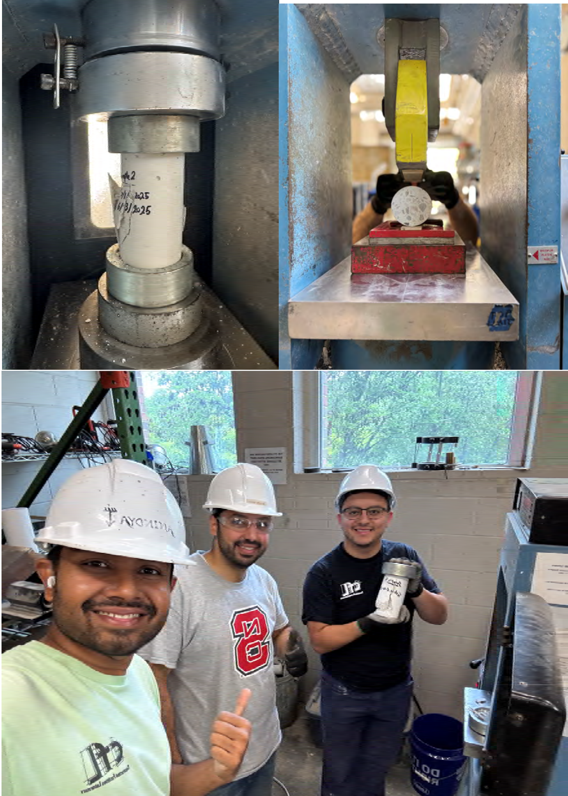
Compressive and Splitting Tensile Strength Tests
