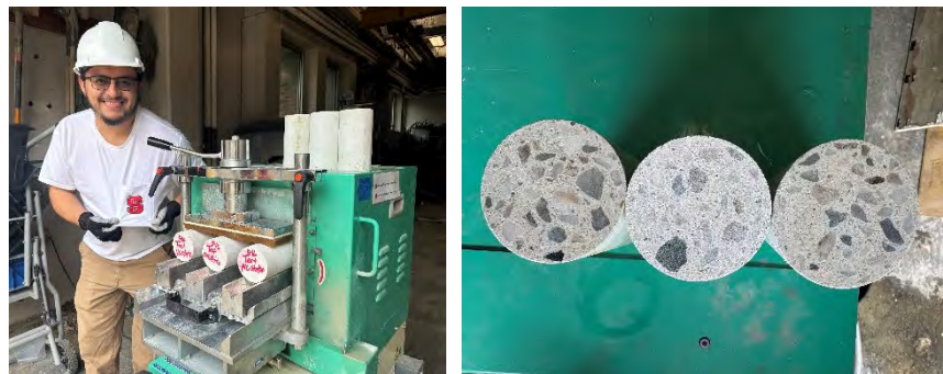
Figure 5: Grinding cylinders for compression testing
