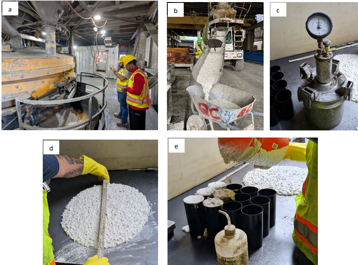
Figure 4: a) Batching concrete b) Taking a sample for quality control c) Air content meter and unit weight measurement d) Spread test e) Casting 3 in \times 6 in cylinders
